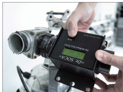
Other than cable tester, it also conduct lamp/load testing.
