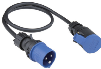
Cable: H07RN-F 3 x 2.5mmsq Connector: 16A 2P+E CEE form (230V)
