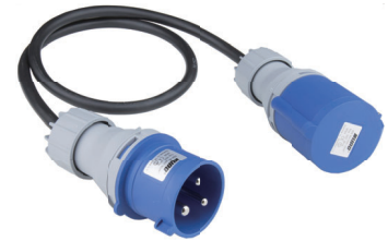
Cable: H07RN-F 3 x 4.0mmsq Connector: 32A 2P+E CEE form (230V)
