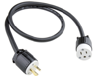
Cable: H07RN-F 3 x 4.0mmsq Connector: NEMA L5-30 or L6-30
