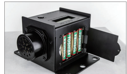
DR.Soca can be used either with 4 x AA Battery.
