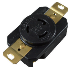
ATL-620R Locking Receptacle Pin: 3 / AMP: 20 / Voltage: 250 NEMA: L6-20R
