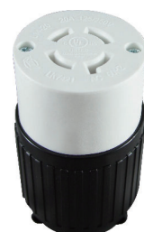
ATL-1420C Locking Cord Connector Pin: 4 / AMP: 20 / Voltage: 125 / 250 NEMA: L14-20C
