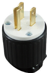
ATL-515P Inline Plug Pin: 3 / AMP: 15 / Voltage: 125 NEMA: 5-15P
