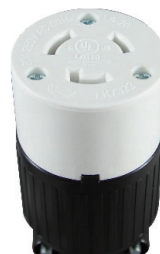
ATL-620C Locking Cord Connector Pin: 3 / AMP: 20 / Voltage: 250 NEMA: L6-20C
